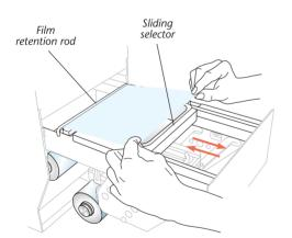
Pull-out drawer for total operating safety, with sliding selector for choosing the desired size of Series
