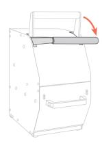
Film sealing cycle with automatic cutting. To start the cycle, simply lower the lever as far as it will go and then release. It will then elevate automatically in a few seconds, after sealing operation has been completed.
