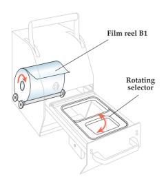
Simple and easy film reel fitting and removal. Simply lay the reel on the rollers once the drawer has been pulled out.
