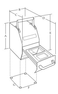
Total weight: 45 Kg approx. (without reel) Power supply: single-phase — earth Power voltage:  $220\ V \pm 10\%$  Power frequency:  $50\ Hz$
