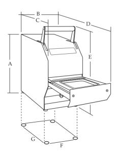
Total weight: 22 kg approx. (without reel) Power supply: single-phase – earth Power voltage:  $220 \ V \pm 10\%$  Power frequency:  $50 \ Hz$  Installed power:  $460 \ W$
