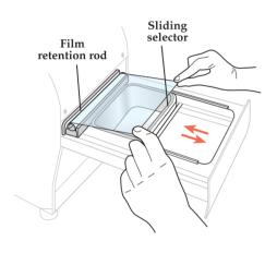
Pull-out drawer for total operating safety, with sliding selector for choosing the desired size of Series P1 - P2 - G containers.
